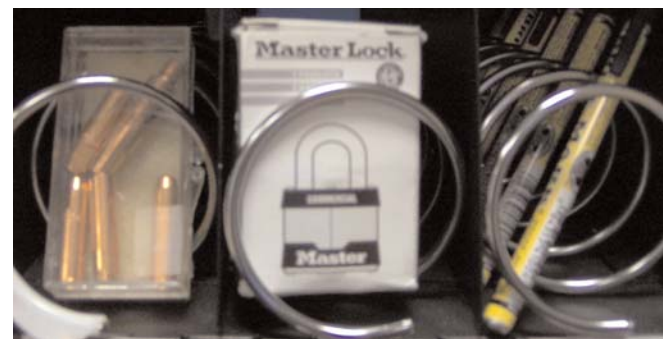
welding tips, locks and brite mark pens dispensed from multiple helix sizes
