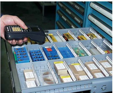
Select the quantity, hit the enter button and immediately log the transaction which adjusts your inventory.
