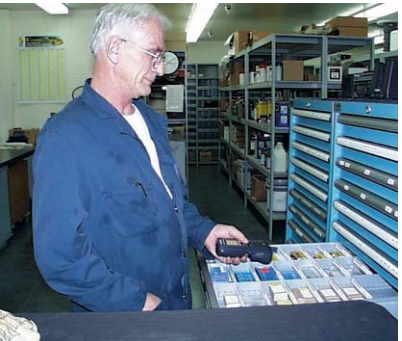
Scan the bin bar-code generated by CribMaster.
