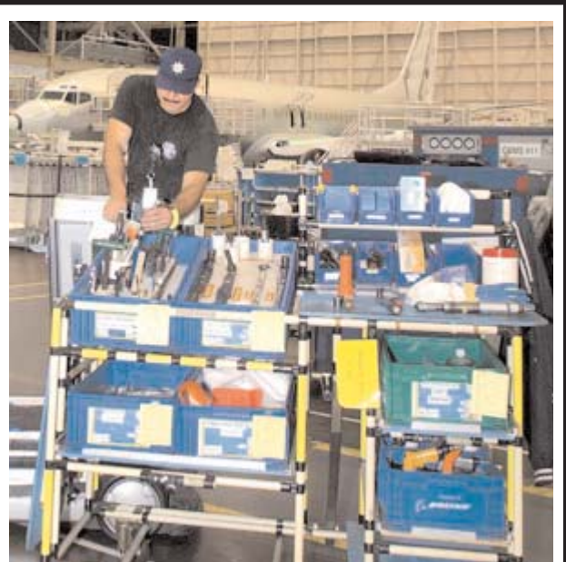
Workers on Boeing's manufacturing-and-assembly moving line have necessary items/tools at their fingertips, but if they do need something, the CribMaster system tells them exactly where it is.
